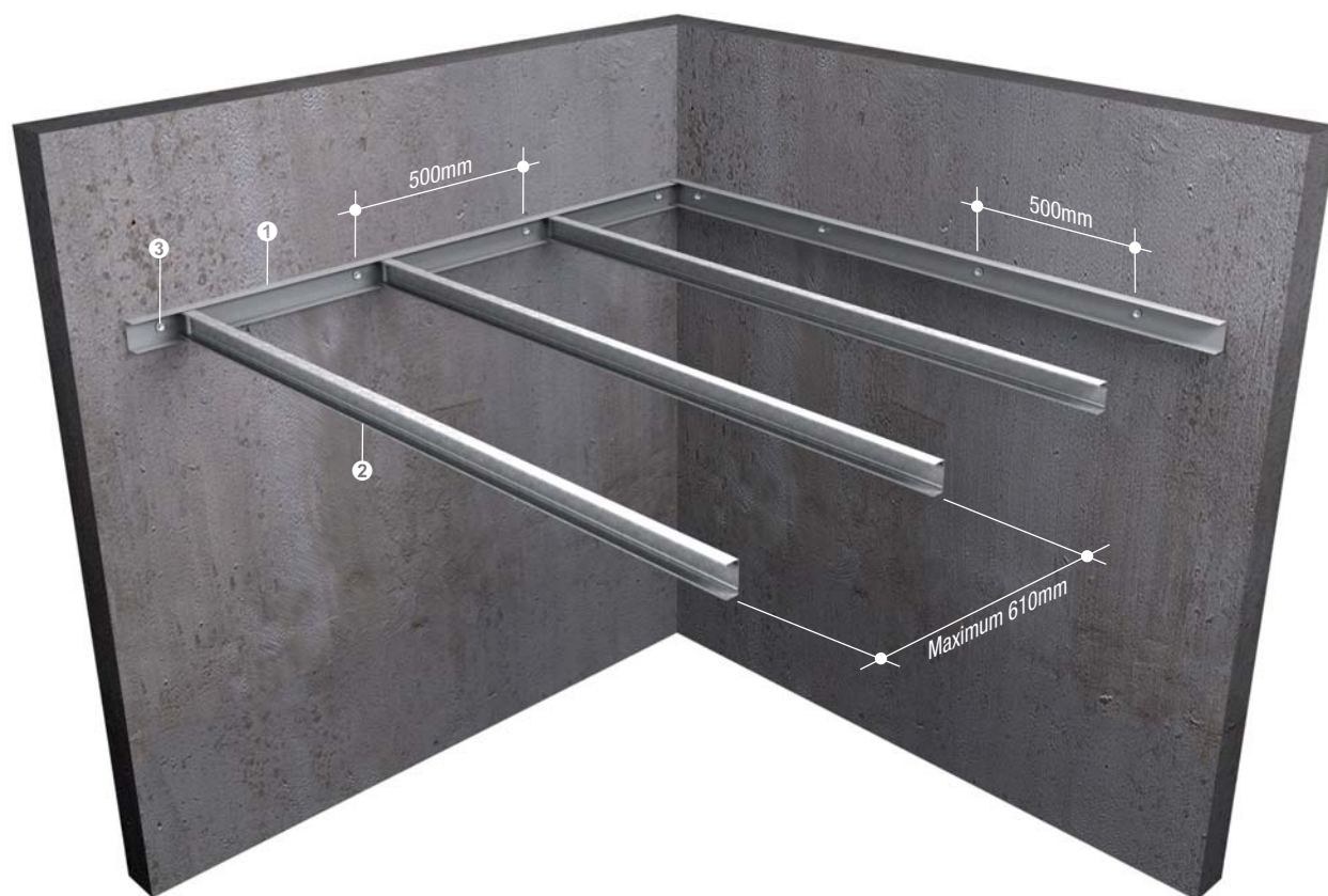
Fixing of primary and secondary profiles
